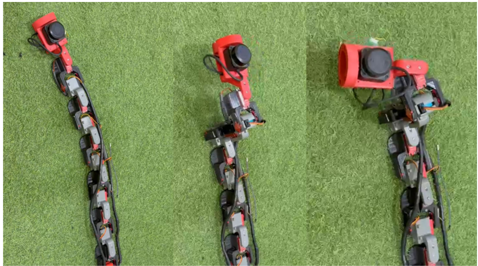
Fig. 14 Execution of the cobra positioning movement from initial rest to elevated scanning posture
